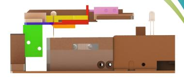
This feeder adds a pin clamping action before the foot cutting action. As shown in the left figure, the pink small cylinder first drives the red pinch piece to fix the pins, avoiding the jumping of the material caused by the orange foot cutting knife. / Pin section deformation and other issues.
