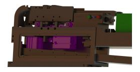
The sports part adopts imported SMC cylinder and NSK bearing With linear guide (pink area above) to ensure material supply The action accuracy and good life of the device
